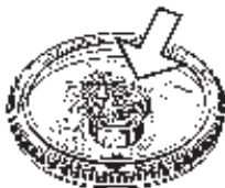
Dosing Capsule while being filled with Magazin Cap (funnel)
