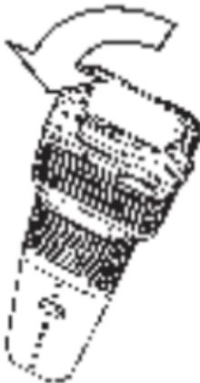
Unscrew the Cooling Unit from the Vaporizer by turning it 90° counterclockwise.
