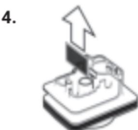
Pull out the Screen inside the Cooling Unit.
