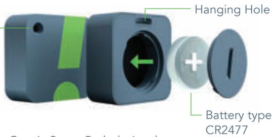
Certain SensorPush devices have a hole or vent in the case for its sensing chip to take readings. Do not cover it.
