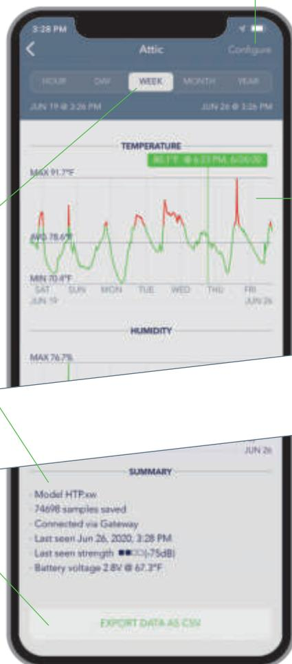
Configure is where you'll find settings for individual sensors, like alerts, sensor name, calibration, etc. See the "Configure Sensor" section of this manual for info.
