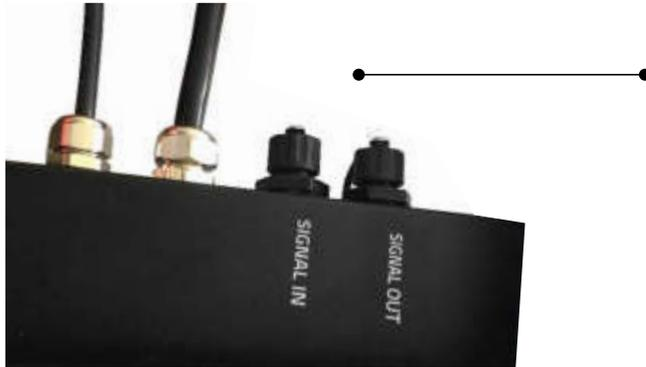
Connect manual dimmer cable or lighting controller cable to SIGNAL IN port.
