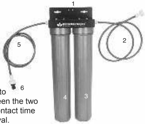
**NOTE:** A flow restrictor is built into the brass connecting fitting between the two housings. This gives optimum contact time for maximum contaminant removal.
