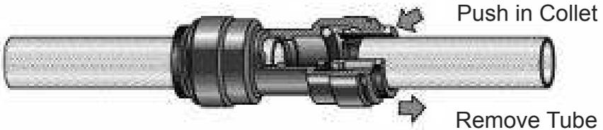
Push tube firmly into the fitting connector all the way to until the tube stops. Try to pull the tube out to check the security. If the tube pulls out, then push all the way in again.
