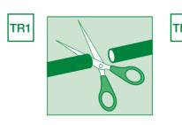
If necessary cut 9mm 3/8" pipe to a length suitable for your setup.
