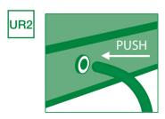
Use a step drill bit to drill a 12mm / 1/2" dia, hole in your reservoir. Push the 9mm / 3/8" grommet into your reservoir. Push 9mm / 3/8"pipe through grommet.
