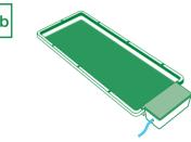
Wet and lay root control sheet on top of capillary matting. The root control sheet can be laid copper side up or down.
