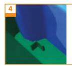
Connect AQUAvalve so 'half moon' is on T section in the trav.
