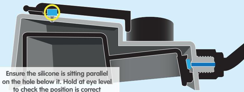
Ensure the silicone is sitting parallel on the hole below it. Hold at eye level to check the position is correct
